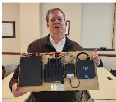
At our last meeting, **Gary Sessums, KC5QCN**, described the portable homemade emergency Winlink transceiver that he built. It's a board-mounted system for VHF communications on 145.630 Mhz with a mini windows PC.
