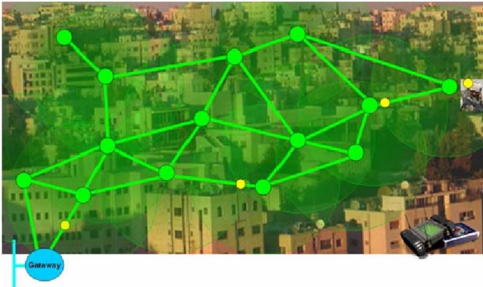
Figure 3 –Self-Configuring Multi-path, Multi-hop Mesh Network Routes Packets (Yellow Dots)
