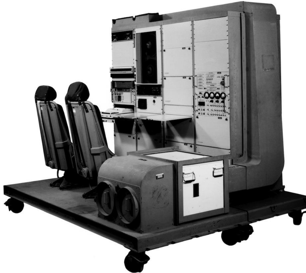
Early 1978-1979 GPS test system for use on the ground or in cargo aircraft.
