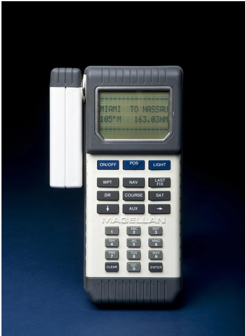
Magellan 1000. The first handheld GPS receiver available to the public. Weight 30 ounces
