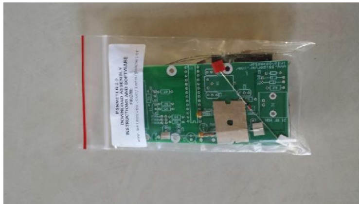
Figure 1 – PSKMeter circuit board kit
